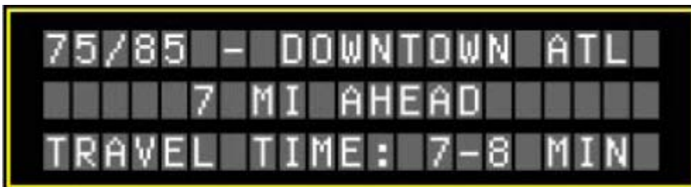
Figure 3.10.1 Example of displaying distance to destination, Georgia DOT
